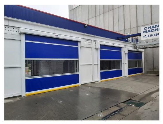
The DMF Series RL3000 Rapid roll door is well suited to carwash applications, and is used to control noise and overspray. Being integrated with the carwash auto control system, the door will close in readiness for the carwash to commence, and then automatically open on completion. A range of door panels and colours is available to suit your needs.
