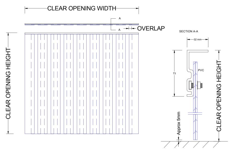
SELECTED VISIFLEX CODE STRIP WIDTH X STRIP THICKNESS X OVERLAP (MM) CLEAR, NORMAL TEMP GRADE STANDARD ALUM EXTRUDED RAIL
